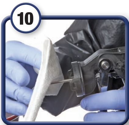
Wipe off any additional residue from the fluid needle.
