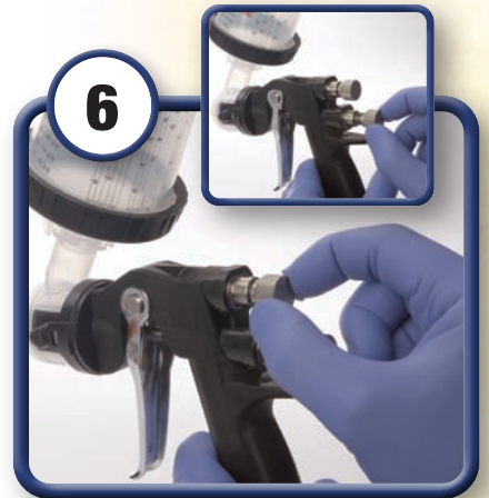
Adjust fan and fluid flow to achieve the desired size and wetness of the pattern. NOTE: when closing the fan adjustment completely it may be necessary to re-adjust the air regulator gauge.
