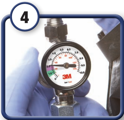
Set air pressure at 2.1 bar (30 psi) for 1 st stage (only air flowing)
