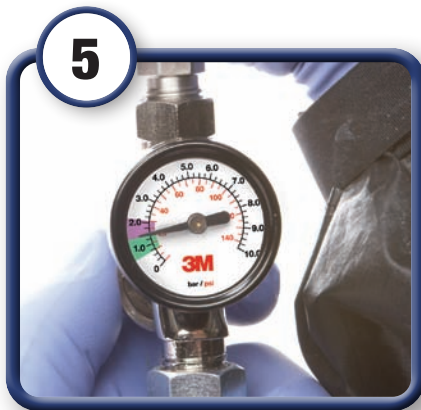
Set air pressure at 1.4 bar (20 psi) for 2 nd stage (air and fluid flowing)
